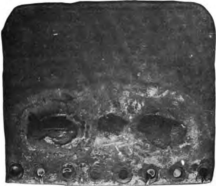
FIG. 5.—A Bagged and Ruptured Sheet.
